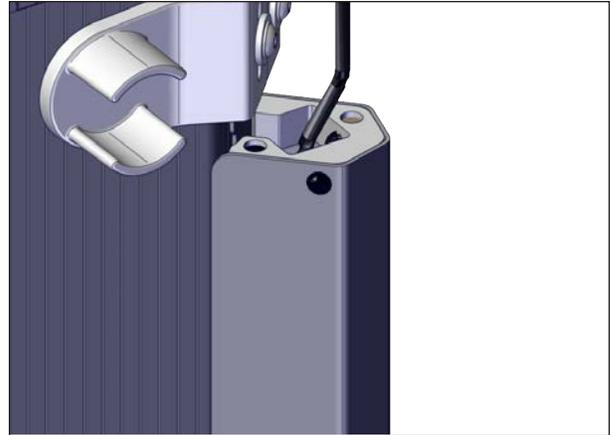
FIGURE 67: CHECK FOR WIRE DAMAGE
